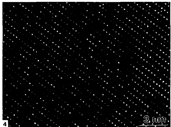
Fig. 4. HRTEM image of \text{Lu}_2\text{Ti}_2\text{O}_7 , with the diffraction pattern of Fig. 3a), demonstrating no modulations.
