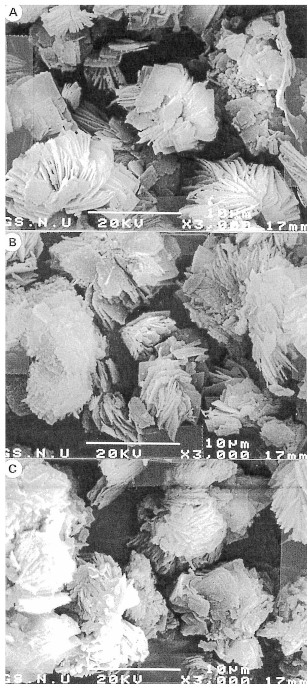
Figure 8. The scanning electron micrographs for the calcined silica-pillared H-kenyaites, hydrolyzed for 10 (A), 20 (B) and 40 (C) min in 0.05 % \text{NH}_3 solution.
