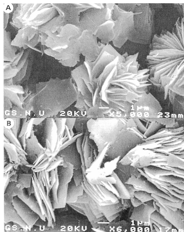
Figure 2. The scanning electron micrographs of Na-kenyaite (a) and H-kenyaite (b).
