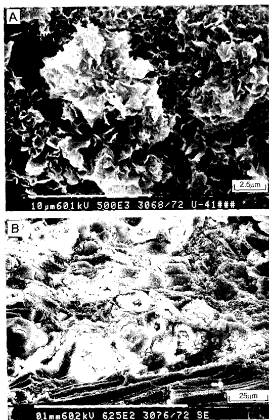
Fig. 5. SEM micrographs showing curling smectite altered from glassy materials (A), and spheroidal cristobalite filled in bubble spaces(B) in a bentonite ore.
