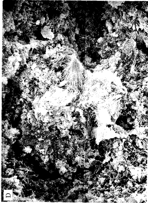
Fig. 7. Photomicrographs and SEM micrographs of zeolites. A : Micrograph showing platy euohedral clinoptilolite grown up in a open space, and smectite replaced from glassy matrix, B : Micrograph showing fibrous mordenite crystallized from amorphous glassy materials, C : SEM micrograph showing lath-shaped clinoptilolite pseudomorphically replaced tricuspid glass shard, D : SEM micrograph showing radial mordenite aggregates grown up in a open space.
