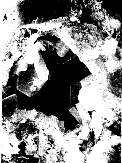
Fig. 7. Photomicrographs and SEM micrographs of zeolites. A : Micrograph showing platy euohedral clinoptilolite grown up in a open space, and smectite replaced from glassy matrix, B : Micrograph showing fibrous mordenite crystallized from amorphous glassy materials, C : SEM micrograph showing lath-shaped clinoptilolite pseudomorphically replaced tricuspid glass shard, D : SEM micrograph showing radial mordenite aggregates grown up in a open space.
