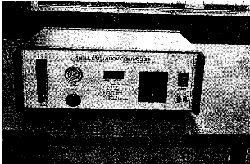
Fig.1. Device for controlling odorant stimulation.
