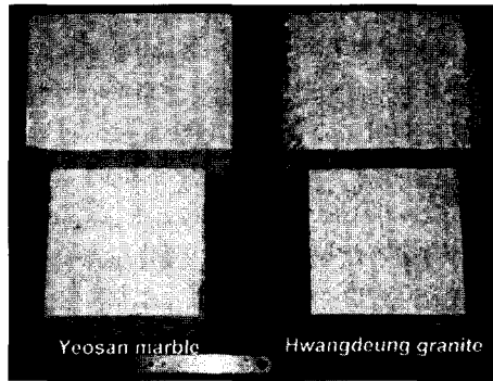
(b) A view of representative fractured joint specimens
