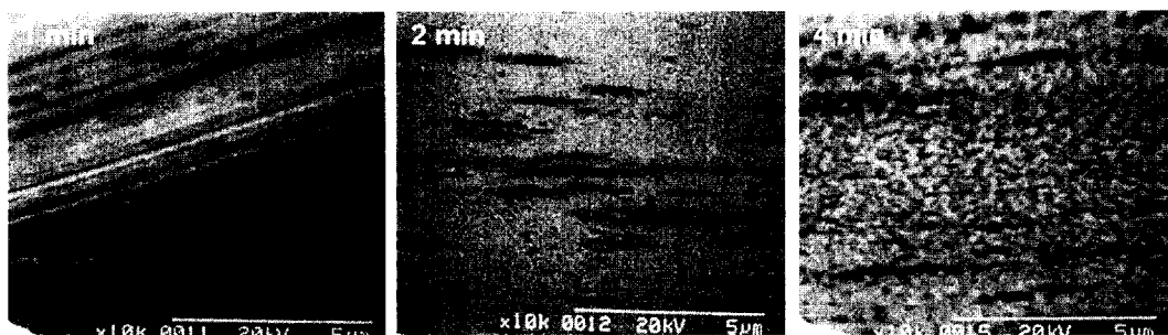
Fig. 3. Effect of etching time with \text{NH}_3 on the surface of Ni layer.
