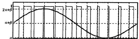
Fig. 1. Basic concept of PWM wave generation.
