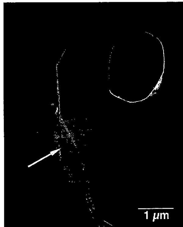
Fig. 5. Dark-field TEM image of damage in the 30.9 \mu\text{m} grain-sized sample deformed \approx 1\% at 1300°C in O 2 .
