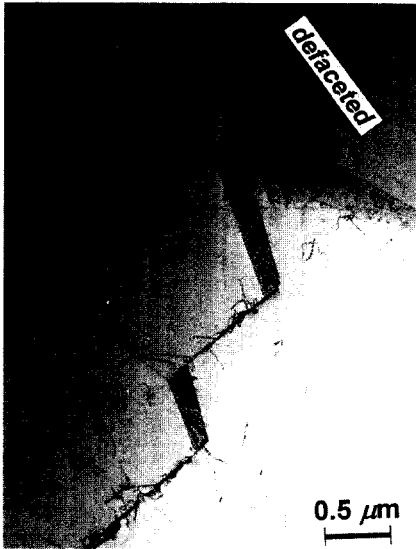
Fig. 1. The TEM micrograph of a faceted grain boundary meeting two defaceted grain boundaries at a triple junction in the carburized Ni annealed at 0.55 T_m for 50 min. 4)
