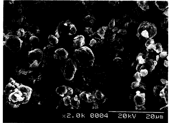
Fig. 2. SEM Micrograph of as-milled MA Ni(Fe)Al-Al 2 O 3 -AlN powders.
