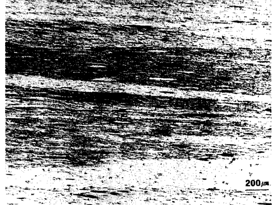
Fig. 10. Optical micrograph showing SRx-like microstructure during simple isothermal annealing at 1350 °C for 1 hr.
