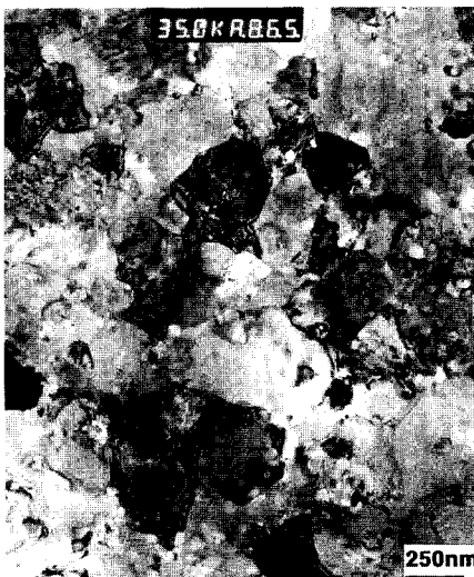
Fig. 6. TEM micrographs of the as hot extruded MA Ni(Fe)Al-Al 2 O 3 -AlN.
