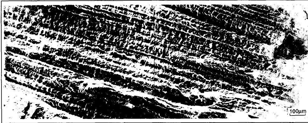
Fig. 4 SEM fractograph of a solidification crack
