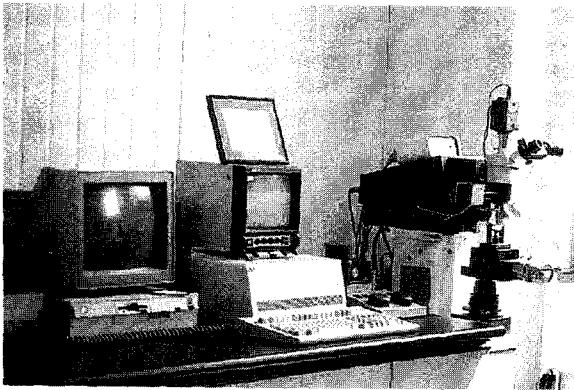
Fig. 2. Monitor and Tukon microhardness tester equipped with a Knoop diamond indenter
