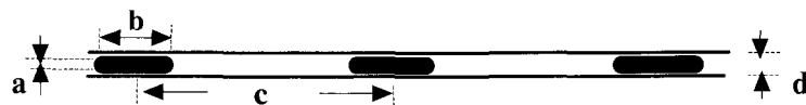
Fig. 2. Fabricated home-made iridium ribbon. a. diameter of source; 0.5 mm b. length of source; 3 mm c. distance between sources ; variable d. diameter of ribbon ; 0.8 mm * Activity; 1~2 mCi for each seed at the time of delivery Strength; 1 mCi/cm ribbon as a standard - 87% intensity of full strength radium needle (0.66 mg/cm)
