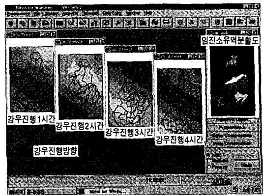
<Fig. 8> Example handling process of radar rainfall data by using raster-based GIS software, IDRISI.
