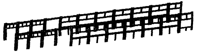
Fig. 19 Side Posts and reinforcements of motorized trailer of TGV-K
