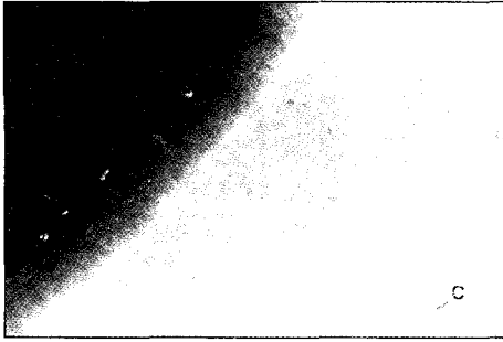
Fig. 8. Definite cell growth inhibition zone was observed around the negative control specimen(Ni)(Magnification X100) (M: Metal, C: L929 Cell).
