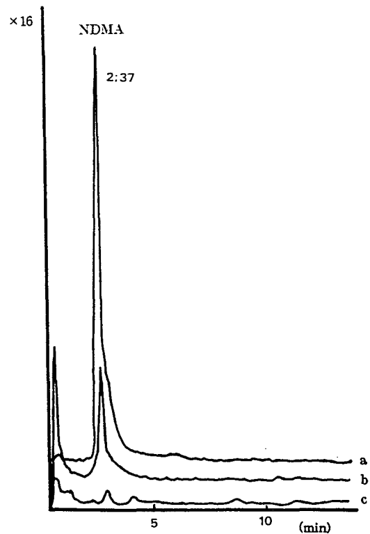
Fig. 1. GC-TEA chromatograms a. NDMA standard 540 ng/ml b. Fermented small shrimp c. UV light irradiated for 3.5 hr. from b.
