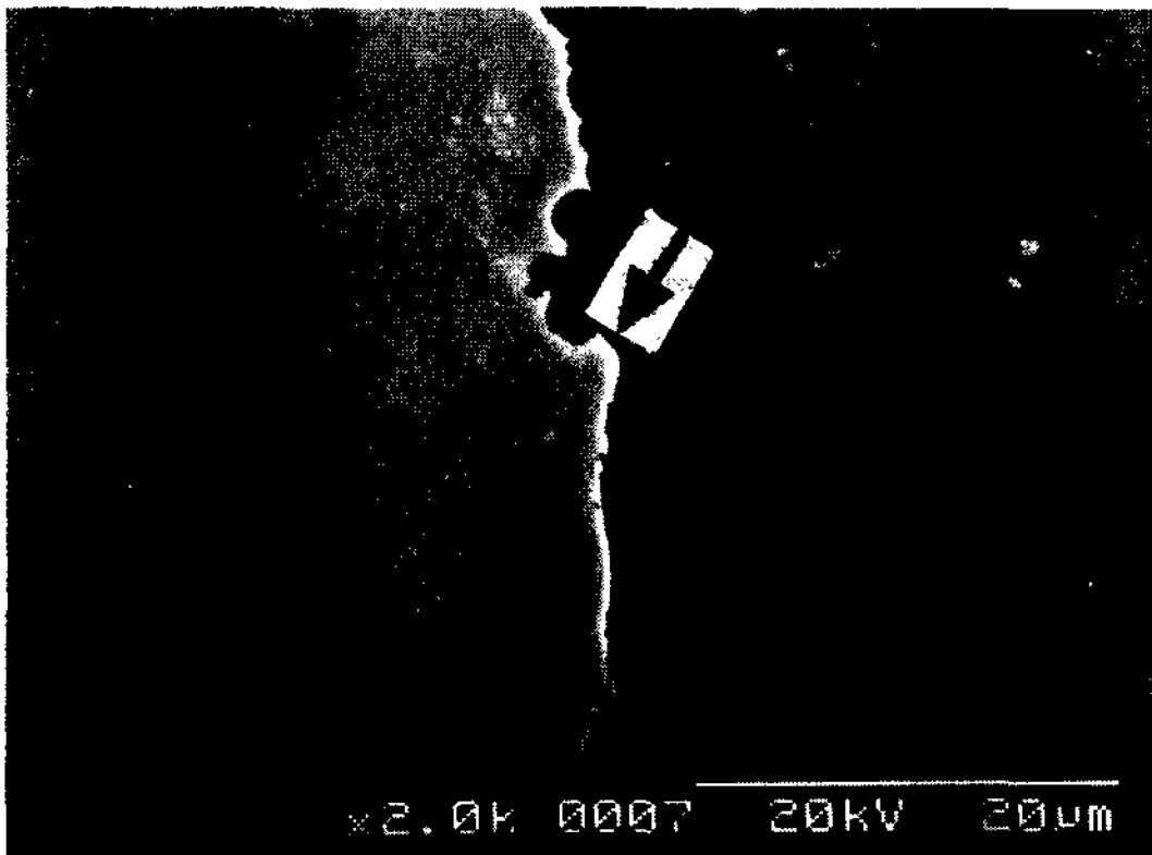
Fig. 6. SEM microstructure at the interface of TiNi/606 Al composite.
