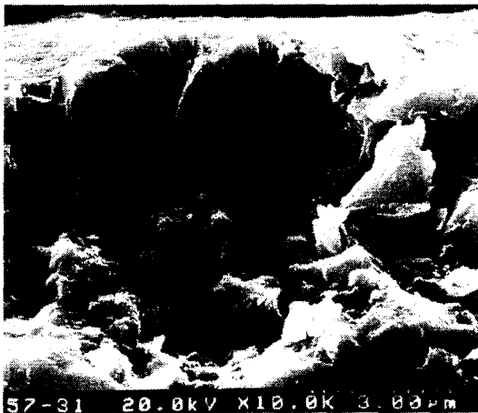
Fig. 2 SEM fractograph on the cross section of coating layer
