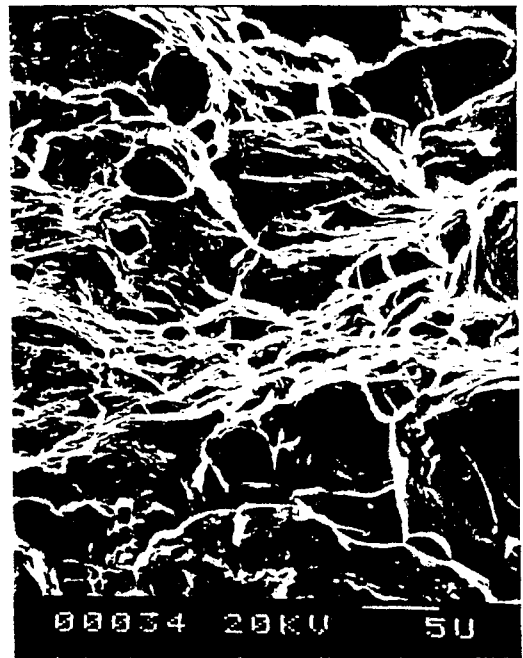
Photo 3 Fracture surfaces of H.A.Z impact specimens at 22°C
