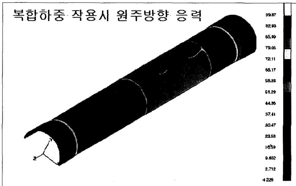
Fig. 9. Hoop stress contour of a cylinder with bracket for combined load
