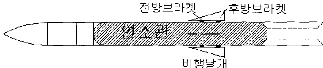
Fig. 1. Configuration of combustion chamber with four fins
