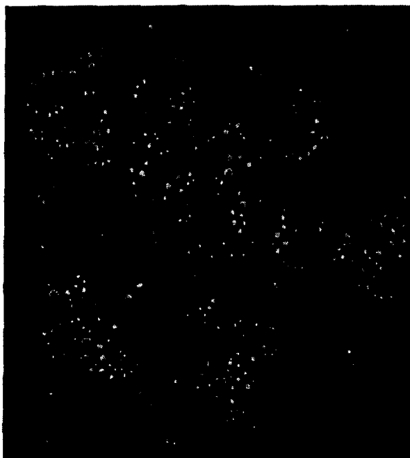
Figure 1. The W/O/W emulsion observed by microscopy and image analyzer. (4.2% of SLES and 0.3% of PGR were formulated) ___400
