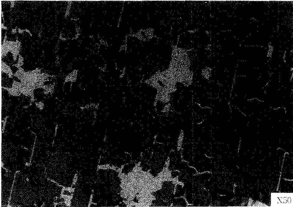
Photo. Optical micrograph of Ti_xN film surface deposited at working pressure ; 4 \times 10^{-3} torr (Ar/ N_2 : 80 : 8), power density ; 9.4W/cm^2 .
