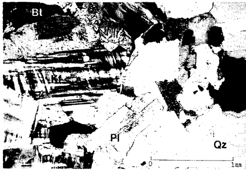
(a) Plagioclase replaced by fine-grained aggregates of clay minerals.
