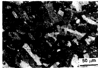
Fig. 2. Microstructure of YBCO superconductor prepared by sintering process[7].
