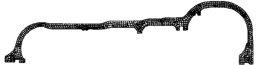
Fig. 13 Finite element model of HP casing of fossil power plant
