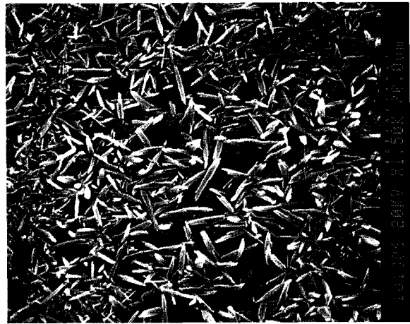
Fig. 4. Crystal growth on the surface of the enamel treated with 65% polyacrylic acid with 0.6M lithium sulfate and 0.3M sulfuric acid for 60 seconds. (SEM X 1500).
