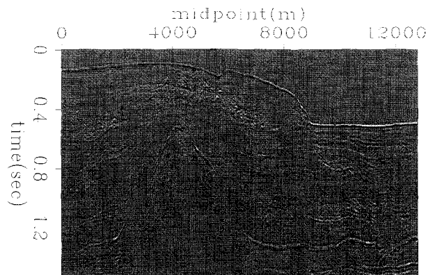
Fig. 10. Gulf of Mexico near-offset data redatumed to the sea level.
