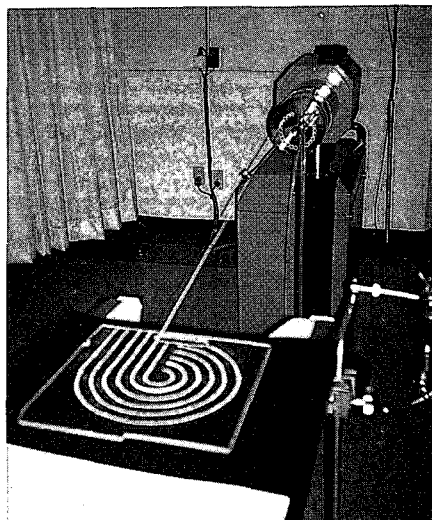
Fig. 3. Source curvature check using source curvature check device
