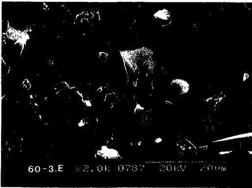
Fig. 13. SEM view of a debonded dentin surface which were slightly air-abraded and acid-etched. Mixed failure mode demonstrate broken resin tags attached to peritubular dentin and the feature of brittle fracture of composite resin on intertubular dentin(X 2,000).
