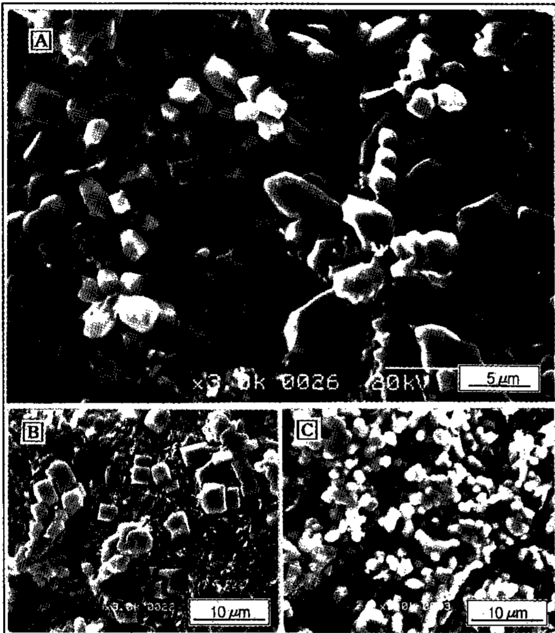
Fig. 9. Dendritic morphologies of TiC in the titanium alloyed layer, etched by HNO 3 +HF+H 2 O solution. A: Typical dendritic morphology of TiC, B: Growth and necking morphology of TiC, C: Grape-like dendrites near the fusion boundary.
