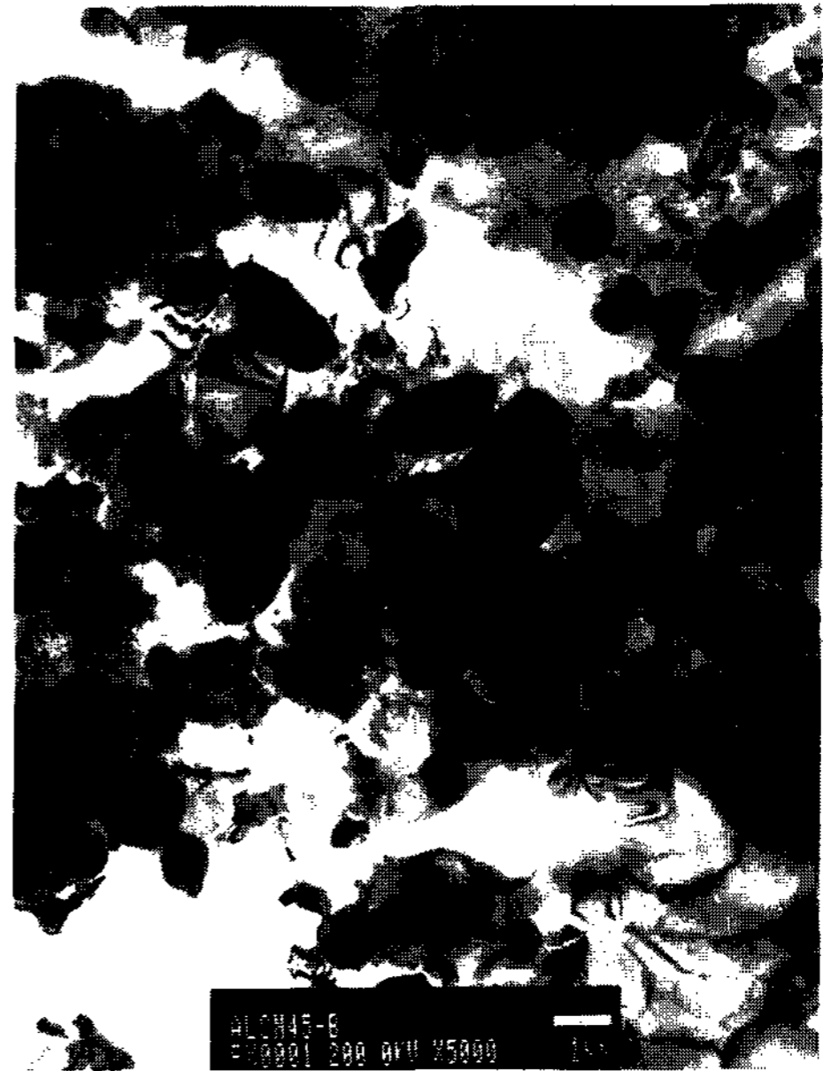
Fig. 7. TEM micrograph of Al_{86}Ni_6Ce_4Mg_4 bulk alloy extruded at 450^\circ C temperatures.
