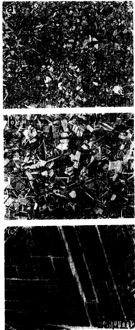
Fig. 1. Optical micrographs of the Fe-18%Mn alloy solution-treated at (a) 700°C, (b) 900°C and (c) 1100°C, respectively.
