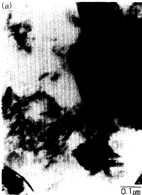
Fig. 3. TEM micrographs of dispersoids in Al-Mg-Mn and Al-Mg-Zr alloys. (a) Al-Mg-Mn (b) Al-Mg-Zr
