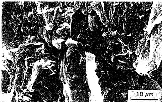
Fig. 10. SEM micrographs of the dynamically vulcanized EPDM and PP/ionomer ternary blends(DCP-0.33phr).
