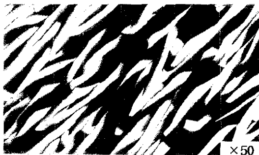
Fig. 4 Surface morphology of WSix/TiW/SC1-cleaned Si annealed in N 2 at 1000°C, for 30min.
