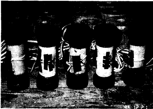
Fig. 4. View of direct tensile specimens of cement mortar.
