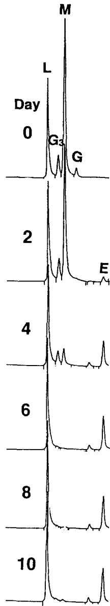
Fig. 2. HPLC of rice Sikhye for wine brewing. Detector, RI Knauer 98.00 ; column, Shimpack SCR 101N ; elution, distilled water, flow rate, 1ml/min. L, limit dextrin ; G 3 , maltotriose ; M, maltose ; G, glucose ; E, ethanol
