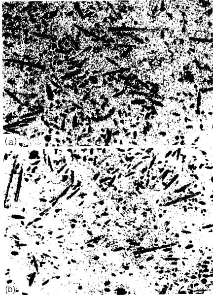
Fig. 5 (a)(b) Optical micrographs for dispersion of Al_2O_3 short fiber on transvse section of hot extruded billet ( S_f=15\% , V_f=15\% )
