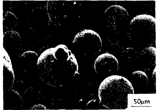
Fig. 1. Scanning electron micrograph of gas atomized D7 tool steel powder
