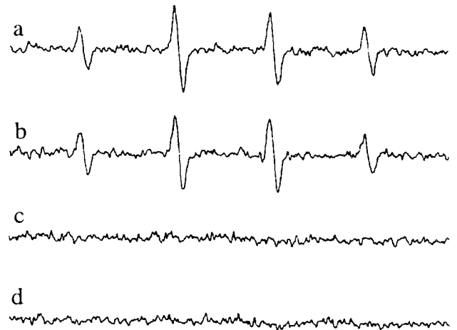
Figure 2. The production of DMPO-OH by NP-III-derived hydroxyl radical under UVA irradiation. The reaction conditions are described in Materials and Methods. The production of DMPO-OH from the reaction mixture (10 mM DMPO + 50 mM NP-III) were recorded (a) under UVA irradiation or (c) without irradiation. Spectra in (b) and (d) show the effect of NEM added to (a) and (c), respectively.
