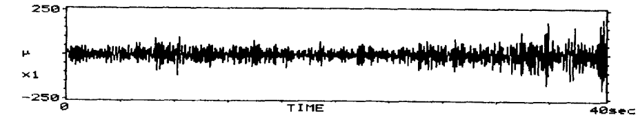
Fig. 15 Measurement result for the horizontal vibration in the EGL conductor roll
