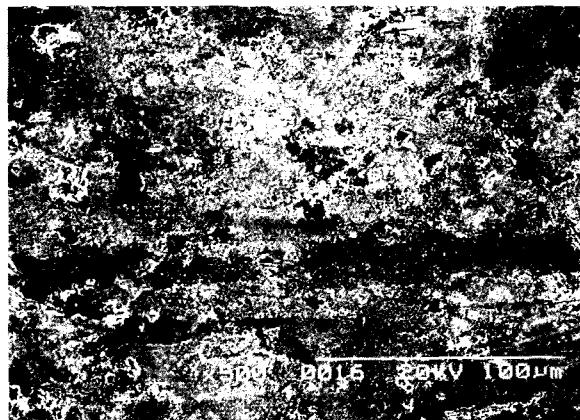
Fig.11. Nickel-chromium alloy surface after tin-plating(X500)
