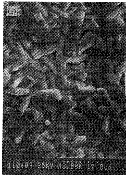
Fig. 5. Secondary electron image of YBa_2Cu_{3-y}Ag_yO_{7-x} superconductors of (a) y=0.0 ; (b) y=0.3 .
