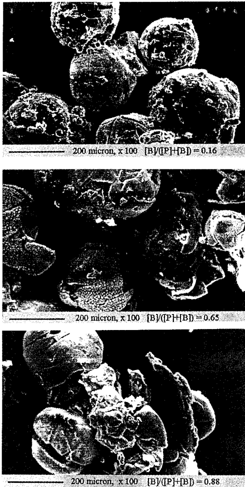
Fig. 6. SEM micrographs of propylene/butene-1 copolymer with catalyst I.
