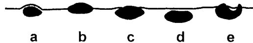
Fig. 10. Hypothetical profile of supper 10 cm of sediment showing levels of nodule burial. a. Nodule from can be seen in photo, but a thin layer of sediment obscures the actual nodule, b. True nodule perimeter is visible in photo. c, Reduced nodule perimeter is visible in photo. d, Nodule shows no surface expression. e. Knobby projections on top of large nodule give the impression of two or more smaller nodules.
