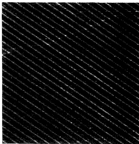
Fig. 1 AFM image of anodic oxide lines fabricated on a Si-H surface. An STM was used for patterning at a sample bias (Vs) of +5.0 V, a reference current ( i ) of 0.2 nA and a tip scan rate ( \nu ) of 0.1 \mu\text{m/s} in nitrogen atmosphere with a relative humidity (RH) of 20%. The region where the tip had scanned protruded 1~2 nm from the surrounding unscanned region due to volume expansion accompanying the anodization of the substrate Si.
