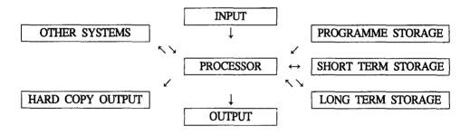
Virtually any computer must have some of these components. In this illustration, OUTPUT and HARD COPY are distinguished although they are often the same thing. In the micro world, however, the basic machine usually has screen output but no printer.
