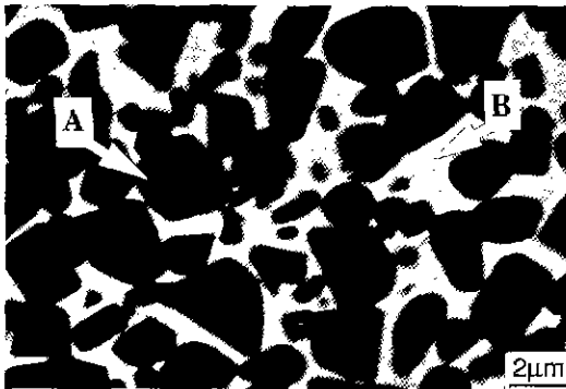
Fig. 1. Backscattered electron image of the reaction-bonded TiC-Ni specimen obtained by the infiltration of the melt with 100% Ni.
