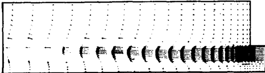
Fig. 7. Velocity vector plot in the furnace.
